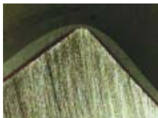
Fig. 2: Poor edge retention of a conventional coating.
