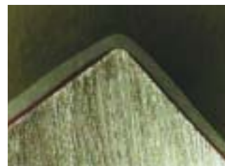
Fig. 3: Improved edge retention of solvent-free epoxy. Photos courtesy of the author.
